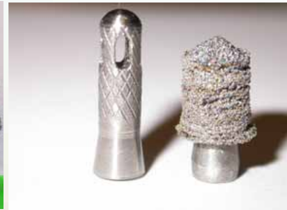
3D level-to-level welding deposition of Ti powder on Ti stomatological pin
